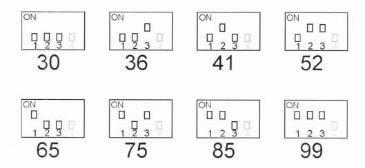
It will be therefore in charge of the system integrator to set the dip-switches according to the speed limit.
